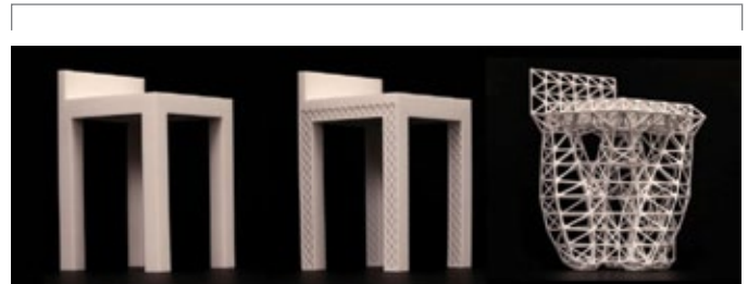
Figure 7: Design Extension for Improved Strength-to-Weight Ratio
