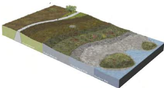
Horizontal Levee (Green + Grey Infrastructure)
