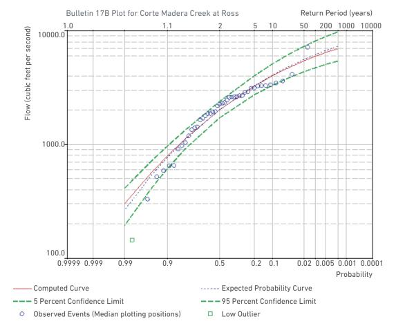
Figure 6. Example Flood Frequency Curve for Corte Madera Creek at Ross in Marin County Source: USGS Surface-Water Daily Data for California
