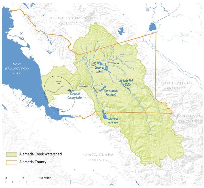
Note: The Alameda Creek Watershed drains approximately 700 square miles, across three counties (Alameda, Contra Costa, and Santa Clara). Three major reservoirs in the upper reaches impound water and sediment and influence the downstream hydrology. Where the watershed drains to the bay, the stream is armored and channelized. Sediment and flood flows that historically spread out over a broad estuary and marsh complex are now contained within the Flood Control Channel.
