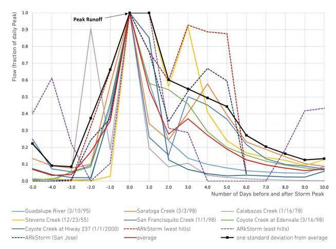
Figure 5. Model Shape Used for Bay Area Extreme Storm and Flood Analysis
