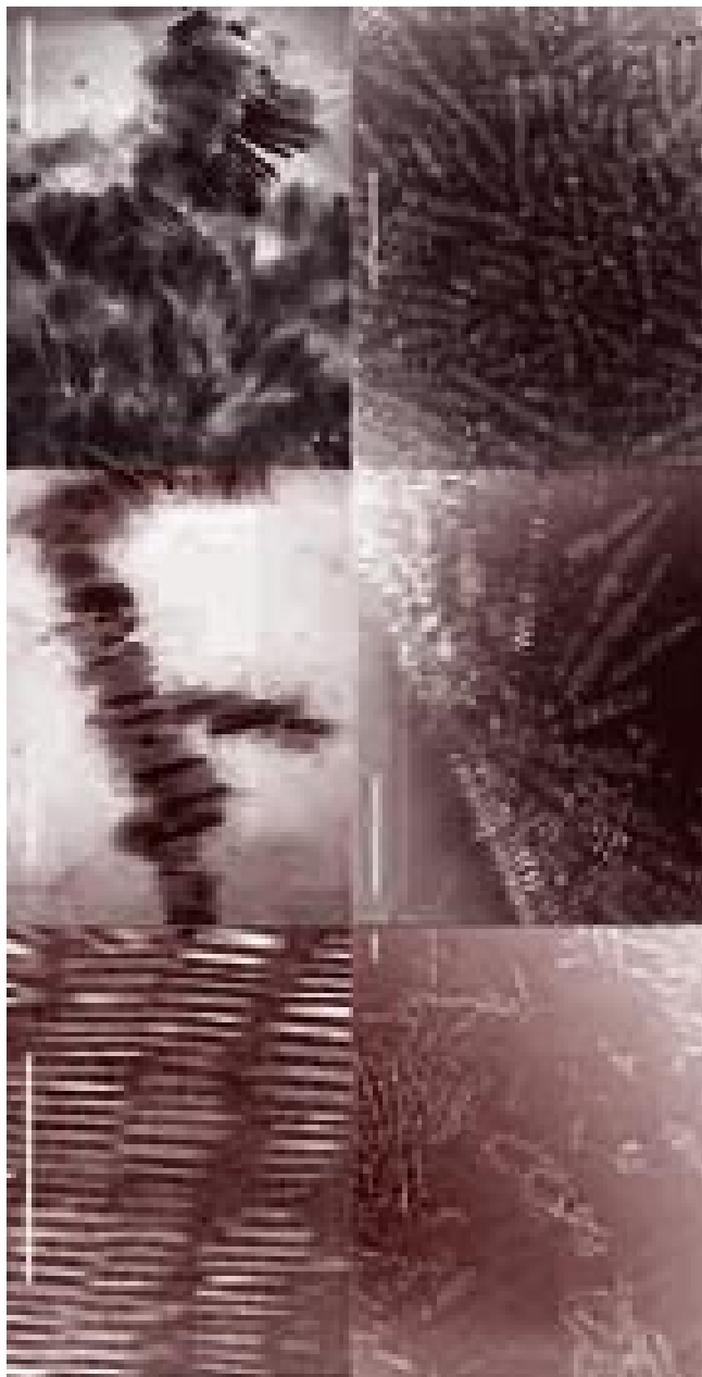
These images show the variety of shapes and sizes that nanocrystals can be made to assume. The rod-shaped nanocrystals to the far left can be stacked for possible use in LEDs, while the tetrapod to the far right should be handy for wiring nano-sized devices. (image courtesy of Paul Alivisatos)
