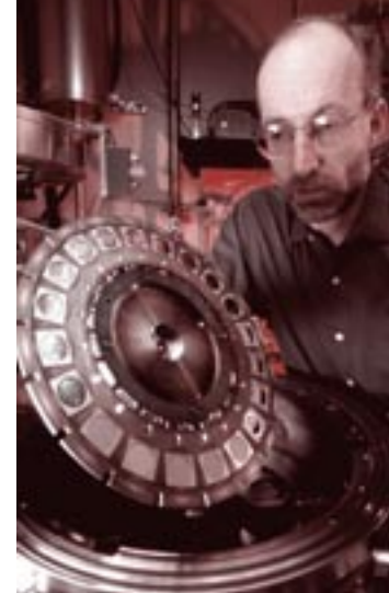
Stuart Parkin, an IBM Almaden physicist, has used a sputtering technique to obtain the GMR effect in materials at room temperature in very small magnetic fields. (images courtesy of IBM)
